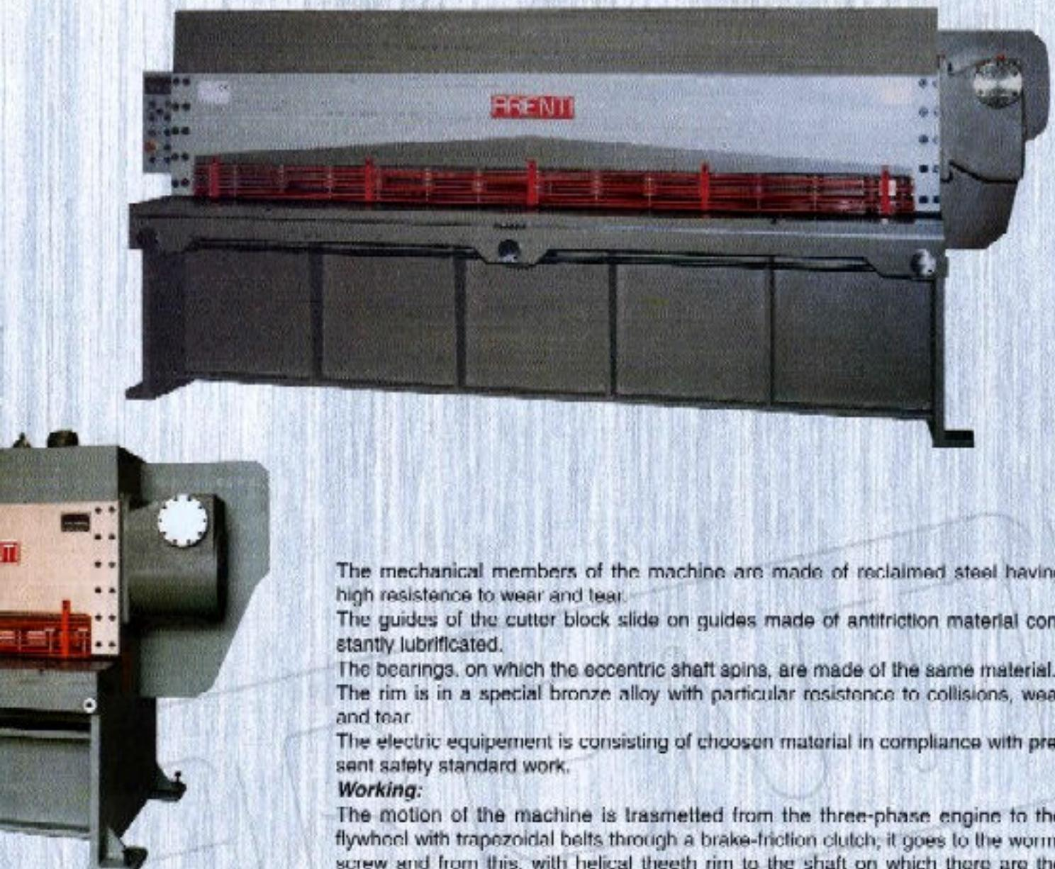
The mechanical members of the machine are made of reclaimed steel having high resistance to wear and tear.
