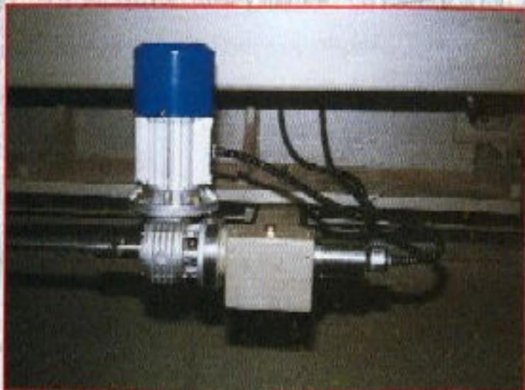
DETAIL OF MANUAL AND MOTORIZED BACK GAUGE
